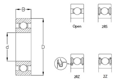
B = 20 Ball grade = 5 C (KN) = 37.1 C0 = 23.2 d = 50 D = 90 Max rpm. = 12000 Type = 6210
